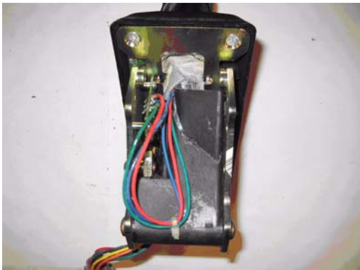
Cracked body inside of shifter
