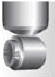
Damaged upper or lower bushing
