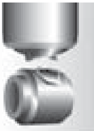
Damaged upper or lower mount
