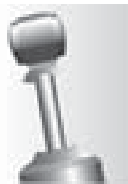
Damaged dust cover and / or shock body
