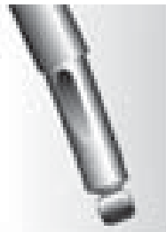
Bent or dented shock
