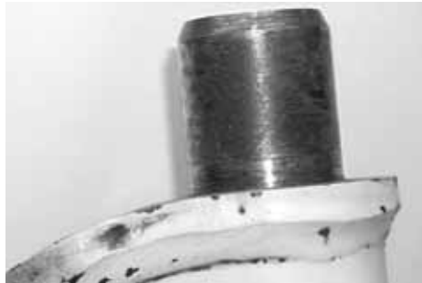
FIGURE 9-50 Kingpin before cleaning
