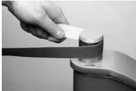
FIGURE 9-50 Kingpin before cleaning
