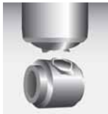
Damaged upper or lower mount
