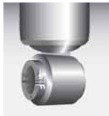
Damaged upper or lower bushing
