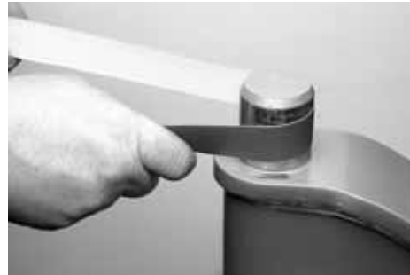
FIGURE 9-51 Kingpin after cleaning
