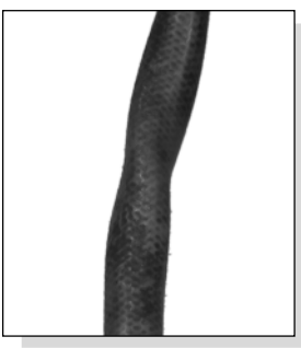
Partly collapsed inlet line shown.
