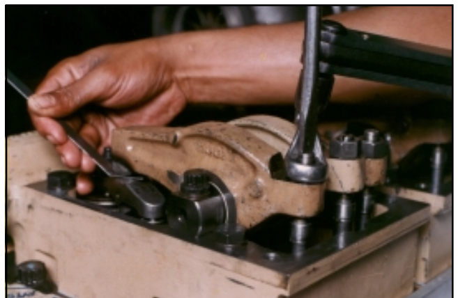
Fig. 7-13. Adjusting crosshead clearance
