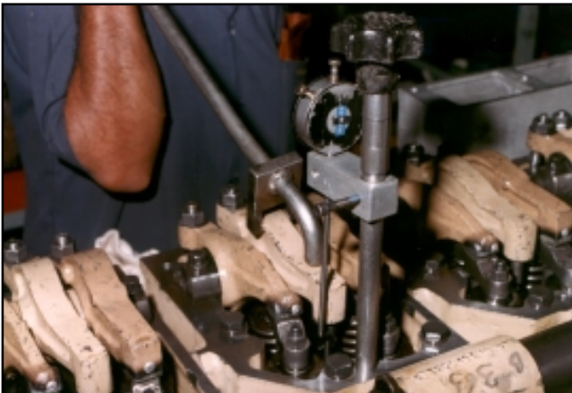
Fig. 7-11. Dial indicator in place—extension in contact with plunger
