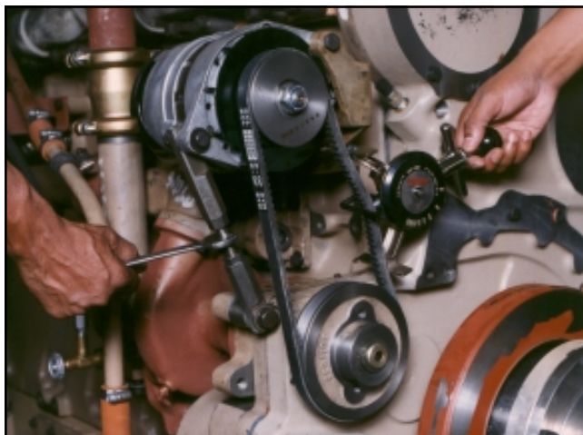
Fig. 4-2. Checking belt tension with ST-1138
