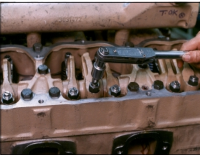
Fig. 7-8. Adjusting injector plunger—V-1710
