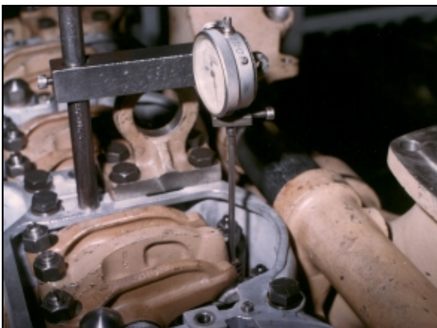
Fig. 7-3. Extension in contact with plunger
