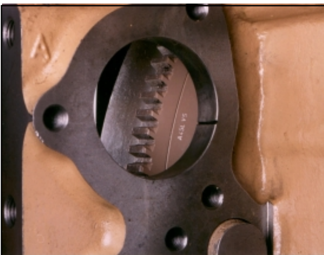
Fig 7-18. Valve set marks on right bank flywheel and housing — KT/KTA 2300
